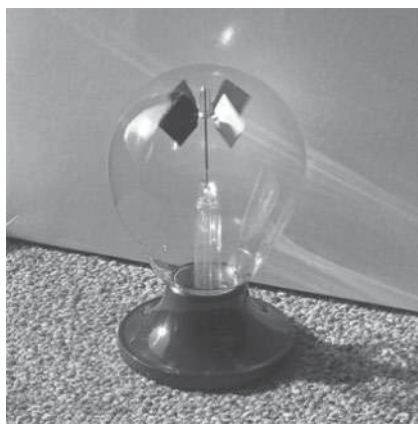
Figure 4.3 Visible or IR light will spin a Crookes radiometer.
